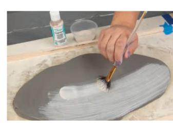
Apply 3 coats of a light colored Cover-Coat® to the slab, making sure that each coat is dry before the next is applied.
