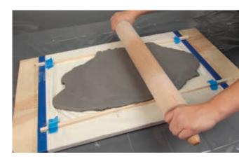
1 Place the 2 boards parallel to each other on either side of the clay so that the slab can be rolled to an even thickness.
